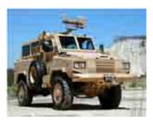
**Specifications.** Protection from Mine/UXO/IED Blast, Ballistic Protection, High Protected Mobility, 4x4 Configurations, Turret Weapon Mountable.
